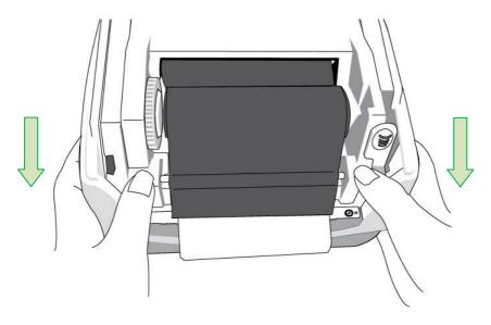
7. Rotate Thumb Wheel of Ribbon Pick-up Holder to remove slack and ribbon wrinkle, and to align the ribbon on the spindles.
