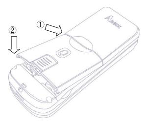
4. Make sure cover is closed and slide two latch back.
