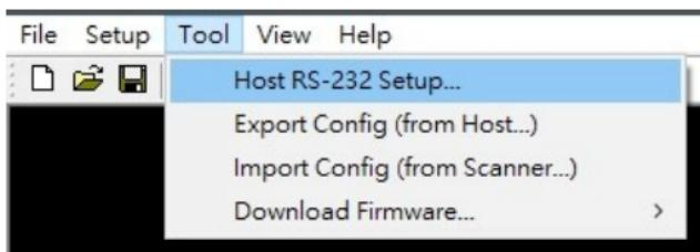
6. In the **Host RS-232 Setup** dialog box, select the COM port your scanner is using and click **Port Setting**.
