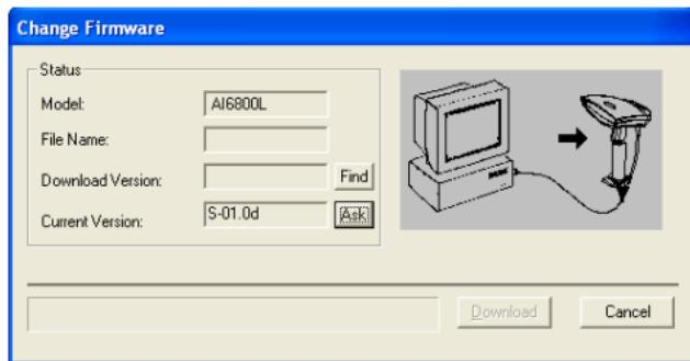
8. Click **Find** to load the firmware file. The firmware version in this file needs to be different from the current firmware version of your scanner. After loading the file, click **Download** to update the firmware.
