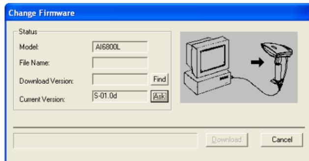
11. Click **Find** to load the firmware file. The firmware version in this file needs to be different from the current firmware version of your scanner. After loading the file, click **Download** to update the firmware.
